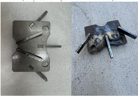
Clamp the bracket against the rotor as shown. Fully seat the narrow concave side against the axle. Make sure the caliper bracket is parallel to the rotor and spaced properly using the press in gussets.
