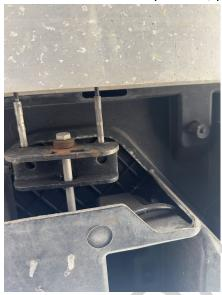
Assemble the master cylinder mount as shown. Note, the master mount balance tee bar is not symmetrical. Be sure to have the outer holes with the small side facing the cylinders. The center hole the small side should face away from the cylinders.
