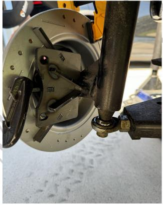
Remove any burrs. Gussets should be fully seated and fully flat against the rotor. The caliper requires the bracket be mounted with 1mm or less tolerance. Tack weld. Test fit, attach a caliper with M10x25mm flange bolts without pads. Make certain the caliper clears the rotor evenly on all sides. Adjust the bracket as necessary before fully welding. The caliper should not touch the rotor at all when it is correctly positioned.
