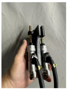
We recommend lengthening the typical master cylinder reservoir hoses up to 36" before install. The hoses can be shortened later but this will let you install and have plenty of length to work with.
